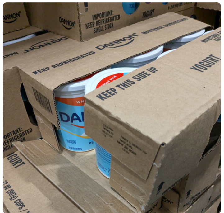
Figure 4: Secondary packaging failure due to box design and/or insufficient glue on the flap.
